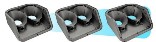
Supplies after unpacking RH80% environment Placement of 1-day printed model
