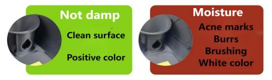
\*The model shown is a display of a common filament material under moisture. The color and brushed state of different filament may vary, so please refer to the actual situation.
