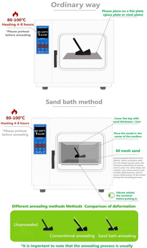
\*It is important to note that the annealing process is usually accompanied by shrinkage and deformation of the model, so you need to be careful in choosing whether or not to anneal the model.
