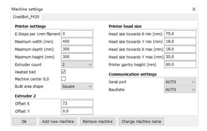
There are alignment problem while printing dual color model, this is because the small difference in multi-nozzle assembly, CreatWare built fine-tuning features.
