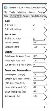
**Solid fill top:** Refers to whether to print the top surface of the model, uncheck will print it with infill method.
