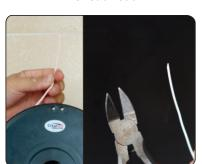
Sharpen and straighten filament head
