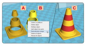
Step 1: Load 2 models you want as shown in figure [A] and [B].
