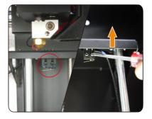
If the nozzle can't touch the platform even loosen all the leveling nut, you can move Z stop limit a little up, as you can see from figure.
